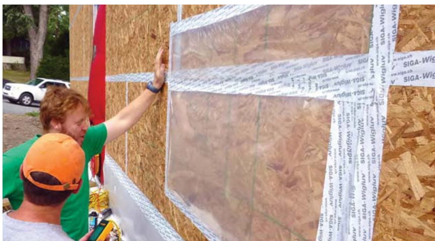
Balloon test #2 over OSB panel only
